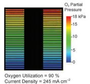
the interior of operating fuel cells can be visualized by using dye films painted on the transparent gas flow field (see image). The spatial and time resolutions are 300 µm and 500 ms, respectively. The oxygen distribution in a polymer electrolyte membrane fuel cell was not in accordance with that expected from the current, suggesting a significant contribution from water.
